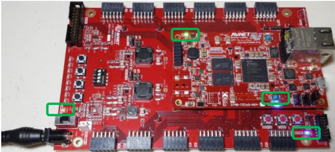
Figure 6 – MicroZed / IOCC Powered On with LEDs
