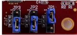
Figure 5 – SD Card Boot Jumper Settings
